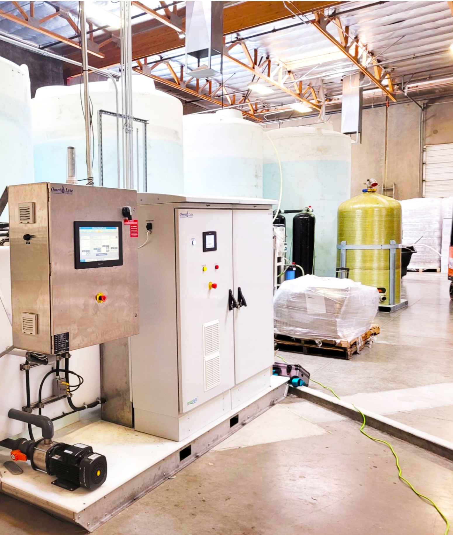
Omnilyte eco12000 alkaline ionized water generator at a bottling plant in USA
